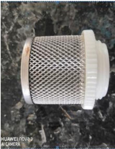
Rotate the suction filter counterclockwise at the bottom and blow the dirt and impurities on the filter screen with an air gun
