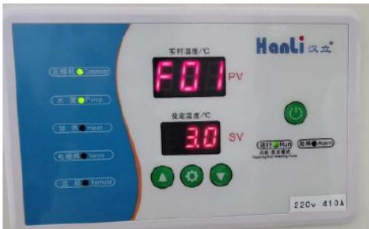
Press setting button to enter the setting, Press the up and down button to adjust the set value, After pressing the set button to confirm the save, press the power button to exit Generally, the default production settings are as followed:
