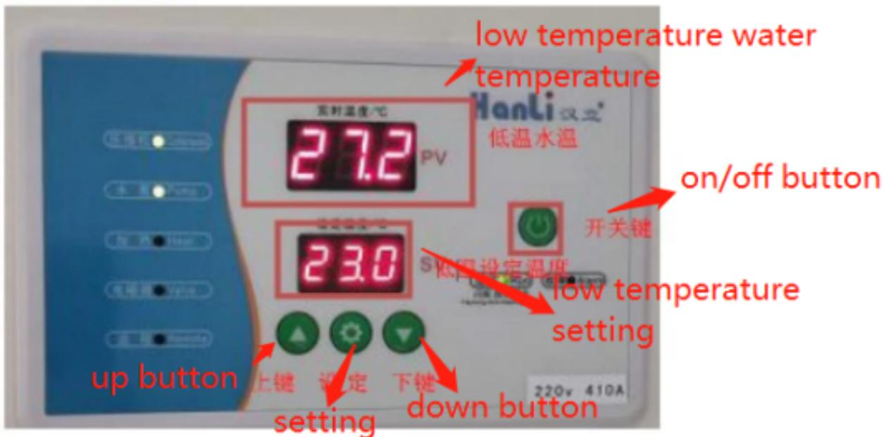
2. Low temperature setting method Press the set button on the main interface, when the low temperature set temperature column is flashing, press the up and down buttons to adjust the set value, press the set button to confirm and save, and press the power button to exit
