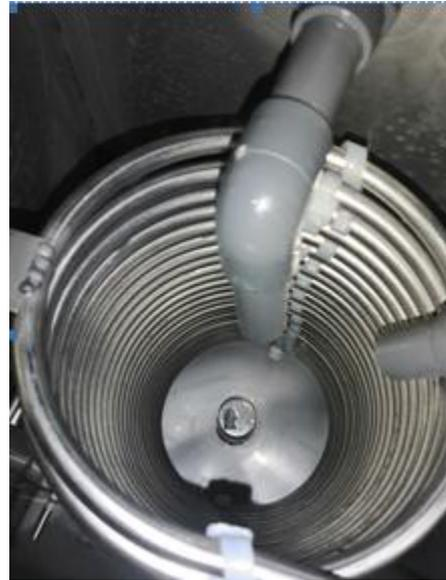
After opening the top of the tank, you will see the suction filter at the bottom of the tank (as shown in the picture above).
