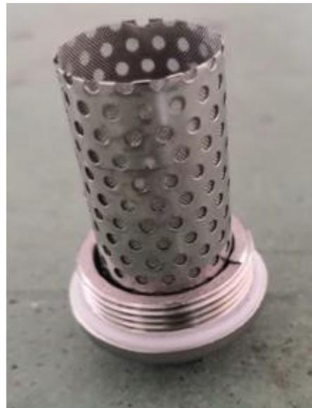
Use the movable spanner to twist the hexagonal counter-clockwise at the lower end of the Y type water filter (need two movable spanners, the left side of the upper go to live, the right side of the counter-clockwise screw down) you can see the Y type water filter inside the filter
