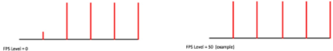
Figure 21: Examples of using the FPS function to control the first pulse suppression.
