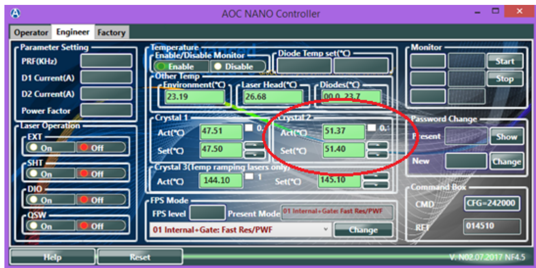
Figure 20: Engineering GUI with Crystal 2 Temperature Section Highlighted
