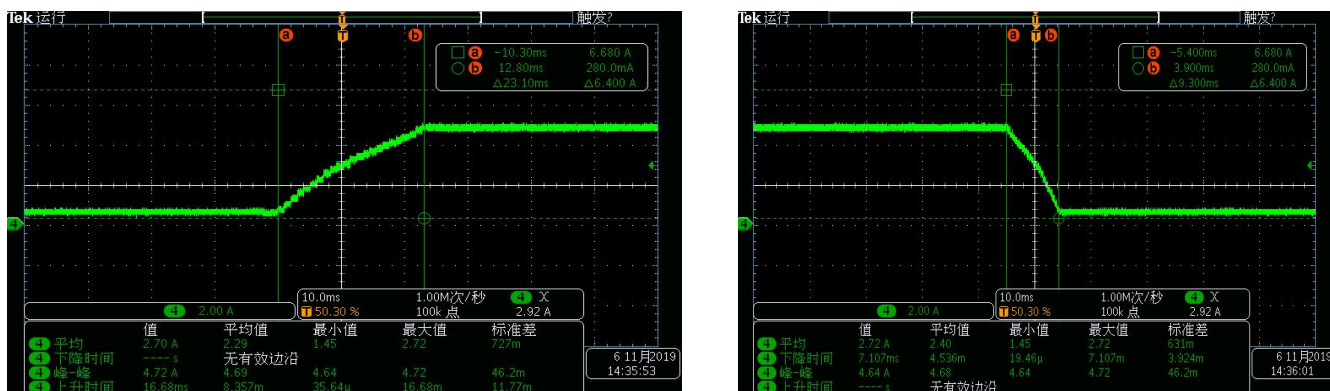
Figure 44 the power slow rise and fall setting area interface and measured programming.
