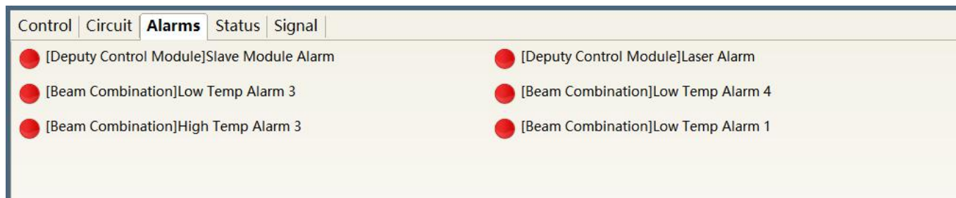
Figure 47 Laser alarm type display area interface
